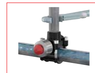
Tighten the bolts crossways. Use the tightening torque specified in the instruction manual. Connect the branch. Make sure there is no water in the branch when the T-plus is activated.
