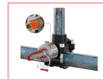
Pull the pin (3). This makes a clean cut in the pipe, creating the branch. And that's all there is to it!
