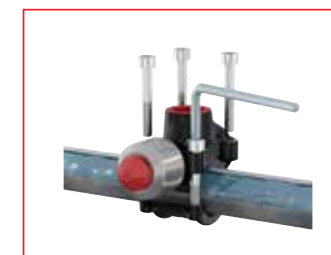
Attach the T-plus to the pipe and secure with four bolts. Models from 1½" are supplied with click-in nuts; the bolt is clicked in, then screwed into place.
