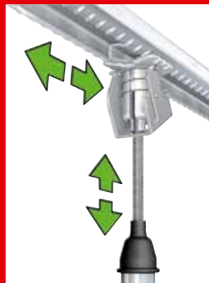
3. Insert the threaded rod into the unit and slide the unit to the desired position. Until the unit is locked by bending the lip, it can be moved freely and the distance from the ceiling can be adjusted.
