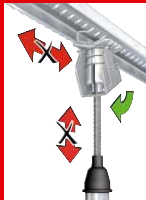
4. Lock the unit. The unit's position in the rail and the pipe's distance from the ceiling is now locked.
