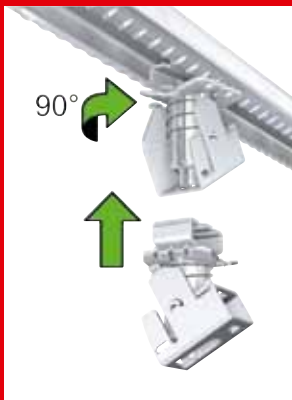
2. Fit the FlamcoFit unit into the rail and twist it into position. The unit cannot now fall out of the rail.
