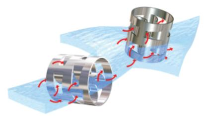
The construction of the PALL ring is such that all the fluid is brought into contact with the total surface of the PALL ring that is available for adhesion.
