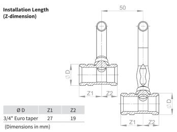
Pay attention to the respective connection dimension (Z-dimension) of the pipe connector used!
