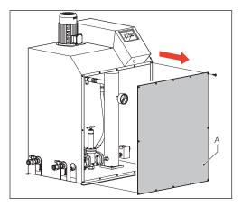
Remove the side cover (A) to gain access to the internal parts. Both left and right covers can be
