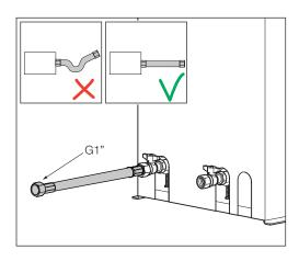
Connect the supply line of the system to the pressure side of the ENA.
